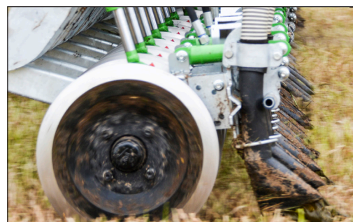
New location of the hose in the cone and new hydraulic pincers
